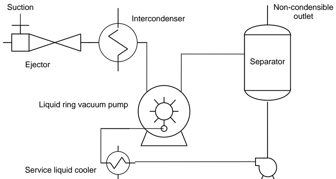
The first stage ejector boosts the interstage pressure to the vacuum pump, thus a smaller pump is required than if the entire compression was to be done by a vacuum pump.
