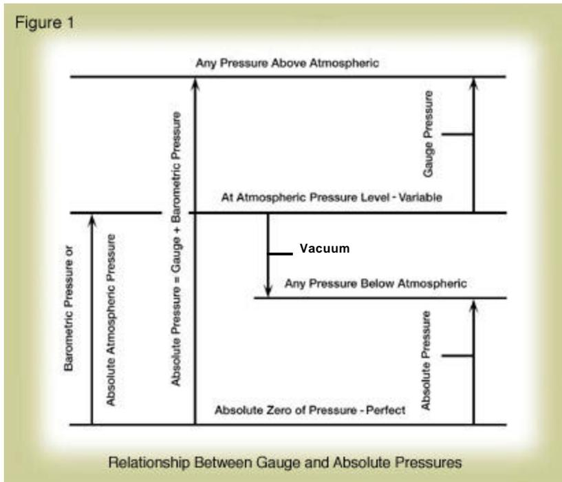
In the prior discussion pressure in a system has been indicated. In order to fully understand what pressure means in the physical world, the following explanation is presented. Vacuum was defined as "complete emptiness". If any gas (or gases) is present in a system a perfect vacuum cannot exist; therefore, by definition, a pressure (no matter how low) will be exhibited.
