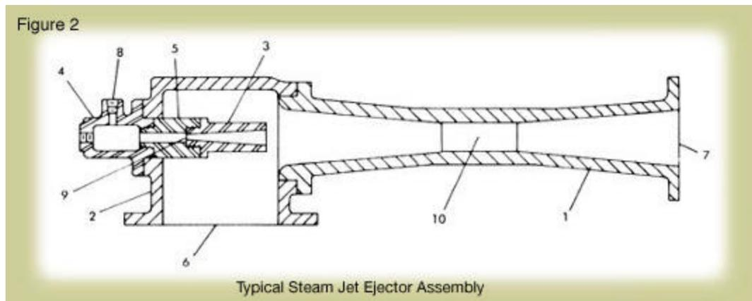
The following describes the basic design and operation of steam jet ejectors.
