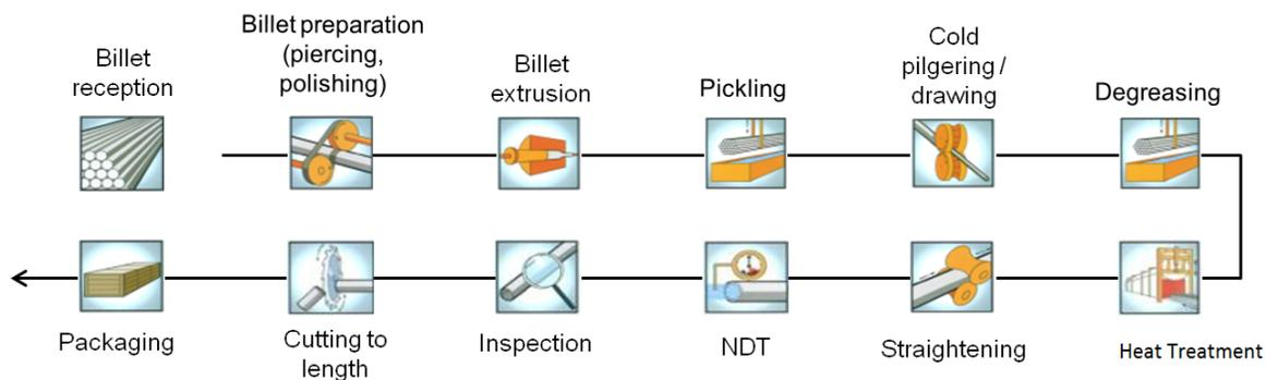
**Typical Process for Seamless Tube Production**
