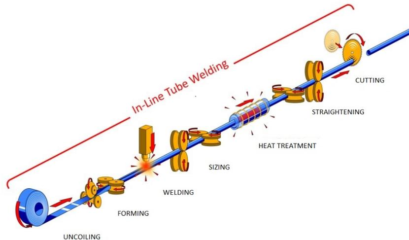
**Typical Welding Process Flow**
