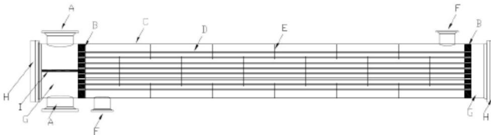
A typical one shell pass, two tube pass, fixed tubesheet heat exchanger.
